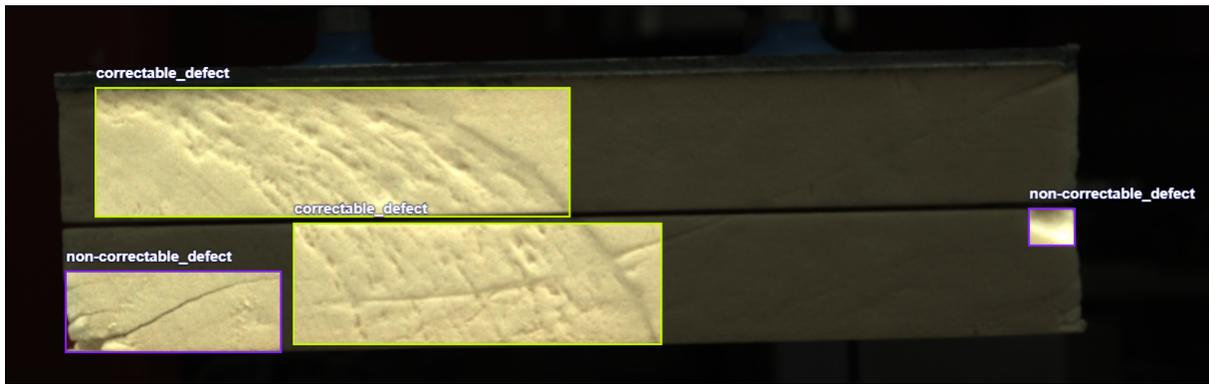
Fig. 4. Item presenting both, correctable and non-correctable defects.
