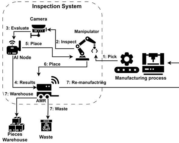
Fig. 1. Quality inspection system description.
