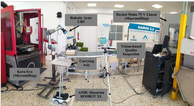
Fig. 2. Manufacturing pilot line.
